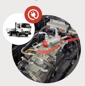
MAZARO's transmissions make current vehicle drivelines exceptionally efficient as they are unique in keeping the engine or E-motor on their best efficiency curve nearly all the time and because they do not contain the usual energy wasters such as clutches, torque converters, synchronizers, piston rings, toroids or belt. There is no traction reduction or efficiency drop during ratio changing.
